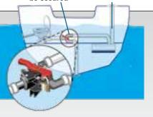
be dumped overboard (for example, any freshwater body of water), these MSDs must have the "Y" valve secured so that it cannot be opened. This can be done by placing a lock or non-reusable seal on the "Y" valve or by taking the handle off the "Y" valve in a closed position.
